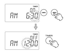
"TIMER" and "OFF" indiactors appear on the display and the "hour" value starts flashing.
